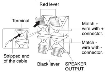
**3** Release the red (and black) lever to close the terminal to fix the cable.
