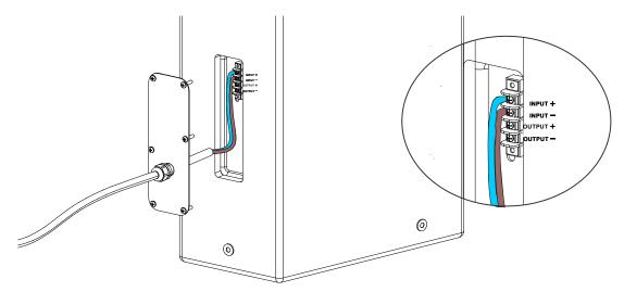
3.- Fix the cover of the rear part of the enclosure with six screws.
