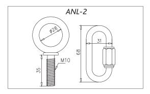
Each ANL-2 eyebolt has a rated working load of 200 kg. (440 lb). Each ANL-2 carabiner has a working load of 330 kg (726 lb). If using other hardware, make sure it is rated to handle the required load.
