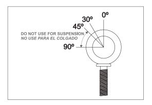
The following illustrations show different views on eyebolt flying for a single box. The length of the back cables or chains determines the vertical angle of the box.
