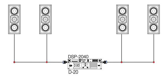
Two WR-8826 (16ohms each) in parallel mode per channel. Refer to the user manual of the D-20 amplifier for SPEAKON connection.
