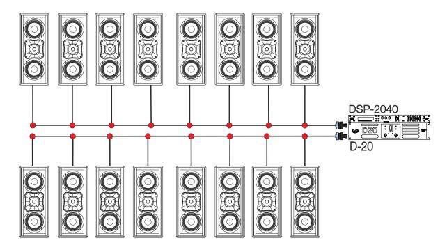
Eight WR-8826 (16ohms each) in parallel per channel. Refer to the user manual of the D-20 amplifier for SPEAKON connection.
