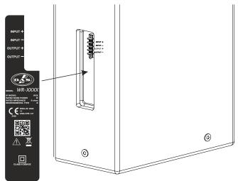
2.- Screw the cables to the barrier strip following the label indications.
