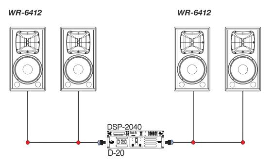
Two WR-6412 (8 ohms each) in parallel per channel. Refer to the user manual of the D-20 amplifier for SPEAKON connection.
