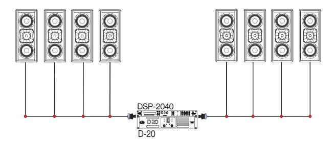
Four WR-8826 (16ohms each) in parallel mode per channel. Refer to the user manual of the D-20 amplifier for SPEAKON connection.
