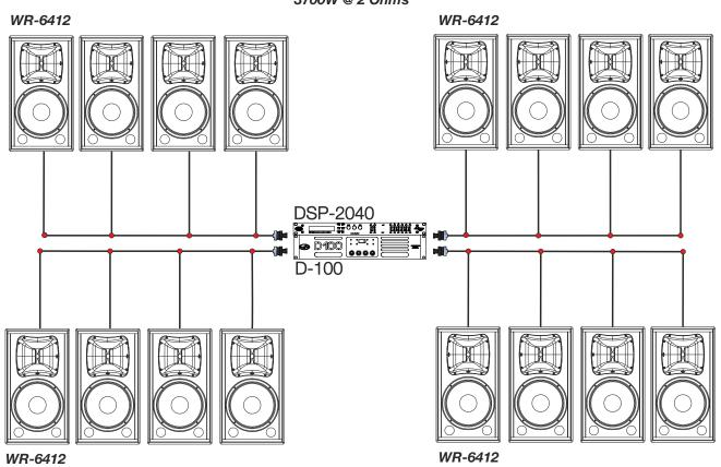
Four WR-6412 (8 ohms each) in parallel per channel Refer to the user manual of the D-100 amplifier for SPEAKON connection.
