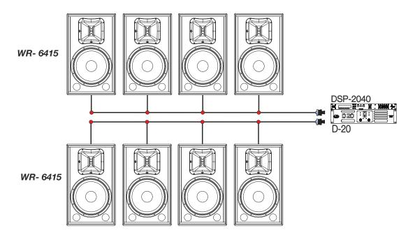
Four WR-6415 (8 ohms each) in parallel per channel. Refer to the user manual of the D-20 amplifier for SPEAKON connection.
