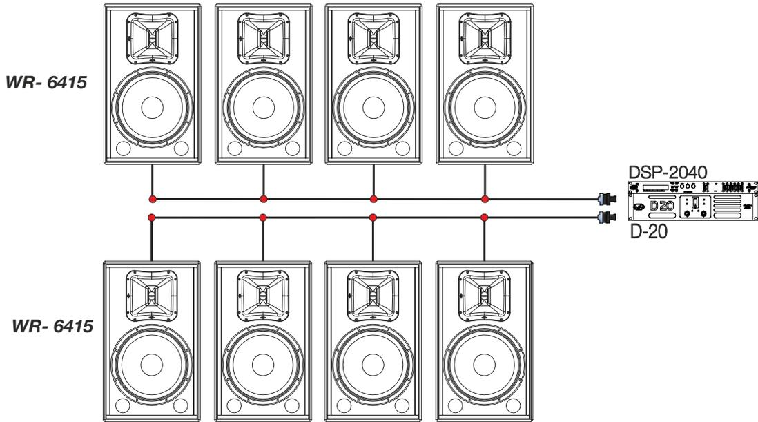
Four WR-6415 (8 ohms each) in parallel per channel.
