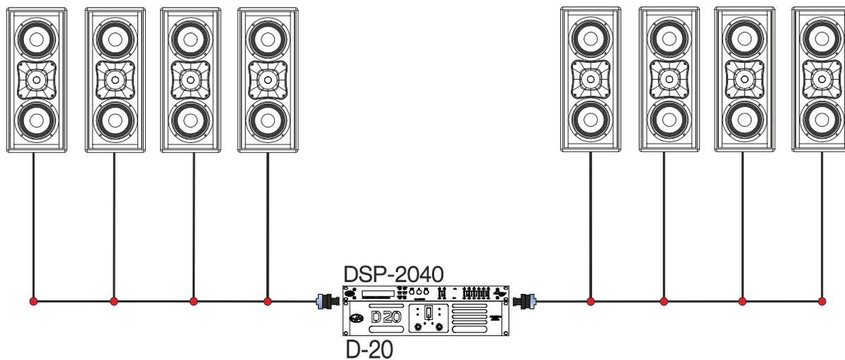
Four WR-8826 (16ohms each) in parallel mode per channel.
