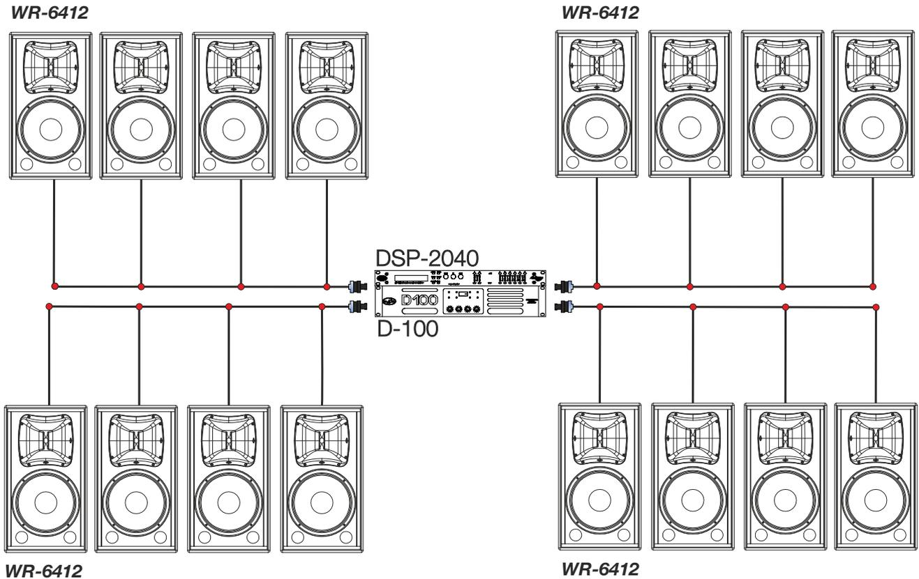
Four WR-6412 (8 ohms each) in parallel per channel
