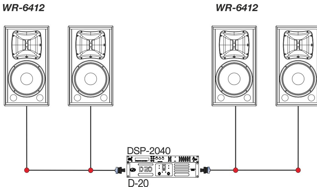
Two WR-6412 (8 ohms each) in parallel per channel.
