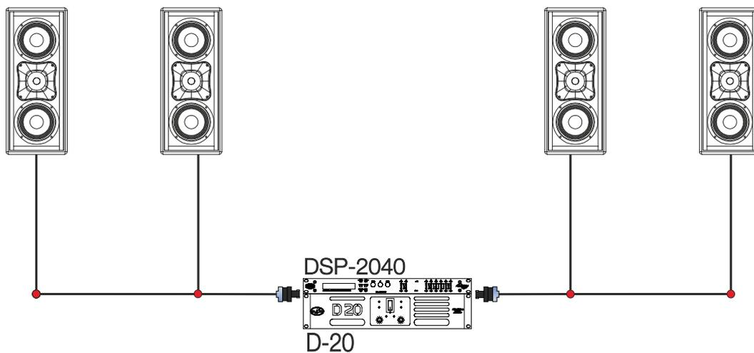
Two WR-8826 (16ohms each) in parallel mode per channel.
