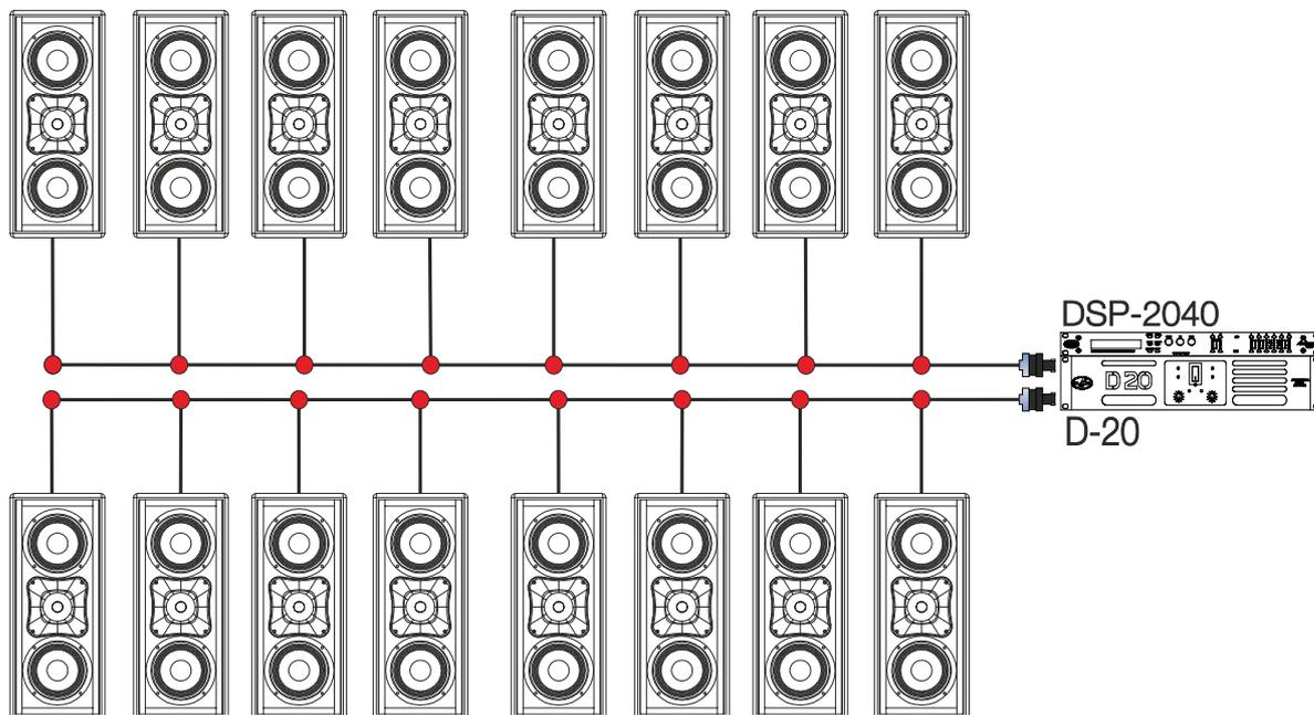
Eight WR-8826 (16ohms each) in parallel per channel.
