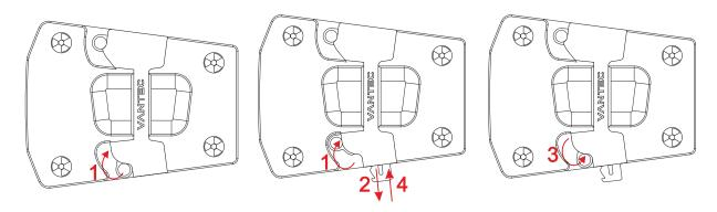
Similarly, to hide the slide we must act on the trigger as in (1) and push the slide up (4), releasing the trigger (3), finally.
