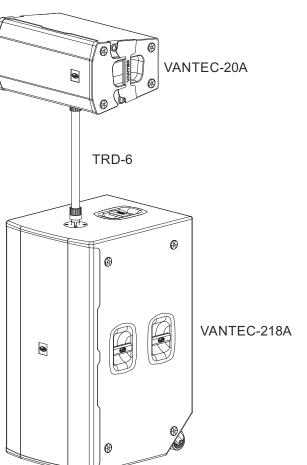
Example of VANTEC-20A on VANTEC-218A with TRD-6
