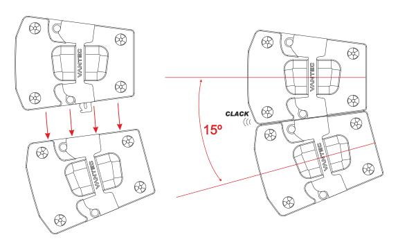
However, if we wanted to unlock the enclosures we would act on the upper triggers of the lower enclosure as indicated below:
