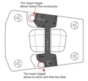
Moving the lower trigger up (1), reveals the slide that will fall by its own weight (2). When releasing the trigger, it will return to its place and the slide will remain fixed (3).
