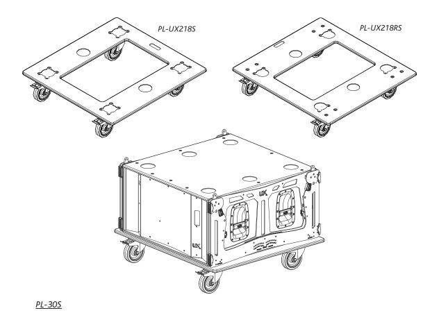
Also a dolly platform is available for transporting and stacking UX-30A units (PL-30S, with WLL = 250 kg). Using this dolly platform we can stack and transport up to two units; and care should be taken to avoid roll over when moving them.
