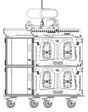
Lift the assembly slightly and remove the dolly platform so as to be able to add AERO-40A enclosures.
