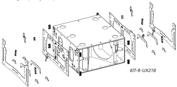
Therefore, only *UX-218A-R* can combine with the *AX-UX218* accessory frame so that enclosures can be flown safely. If an extra pick-up point was needed, a *PICKUP-AX-AE40S3* center bar could be added. This is shared with *AERO-40A* systems, so that *PICKUP-AX-AE40S3* allows for easy combining with these line array systems.
