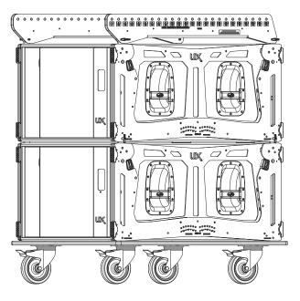
Attach the pick-up point, or pick-up points, to the holes in the side of the AX parts indicated by *Ease Focus*, using the quick release pins.
