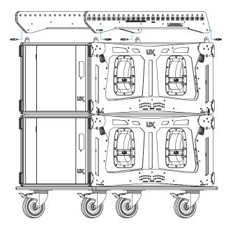
Next, engage the quick release pins to attach the AX parts to the stacked units, on both sides of the units.
