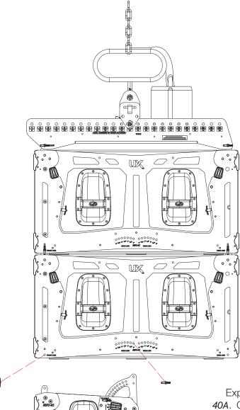
Expose the guides in the upper AERO-40A. Once the guides are prepared and aligned, link the two groups together using quick release pins.
