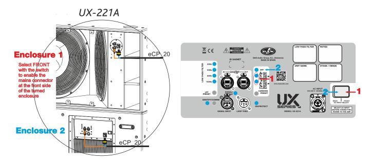
With *UX-221A* units, select FRONT with this switch to enable the mains connector at the front side of the turned enclosure (enclosure **1**), while select REAR for the enclosure **2**.
