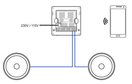
**4ohm** load per channel, BT audio input from a tablet or mobile phone
