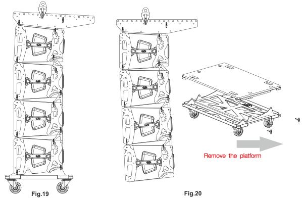
Next, we will place another group of enclosures underneath to continue joining enclosures, and we will repeat the process of angulation of enclosures one by one as indicated above.
