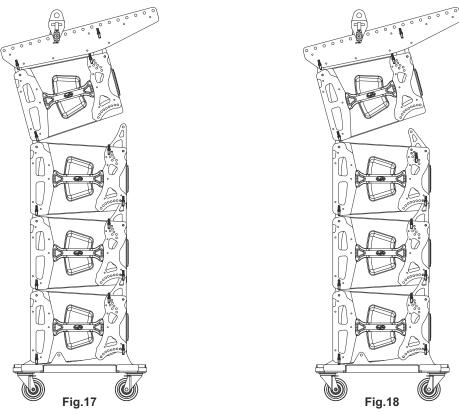
Now we will go down until support the set again, and place the "Rear Link" pin (Fig. 19). This process will continue until all the enclosures have been angled. And finally, the platform will be removed by placing the lid on it again and holding it with its pins.
