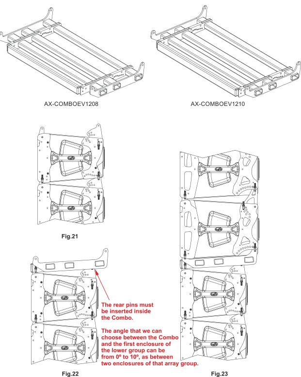
The platform PL-EV212S has more a mission of transport of units (maximum 4 units), than for a stacked use as such, since the angulation of the boxes could make the whole unstable and makes its use for stacked systems not recommendable.
