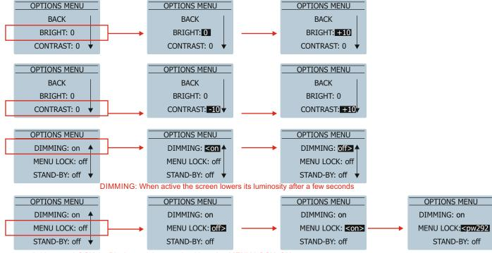
A. User can LOCK the Display and the encoder this option MENU LOCK: ON
