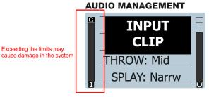
As well, try to avoid excessive volume at the amplifier's output (right signal meter). Be sure that your gain structure is adequate and not causing amplifier LIMIT:
