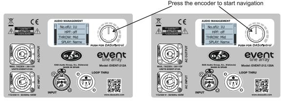
Note: The INPUT and LOOP THRU are type XLR balanced connectors.
