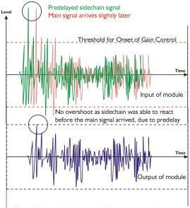
The *DSP-2040*'s "D-Max" limiter predelays the sidechain signal, resulting in a "zero overshoot" limiter, which is able to catch all peaks and provide a reliable absolute maximum setting for the output of any channel.
