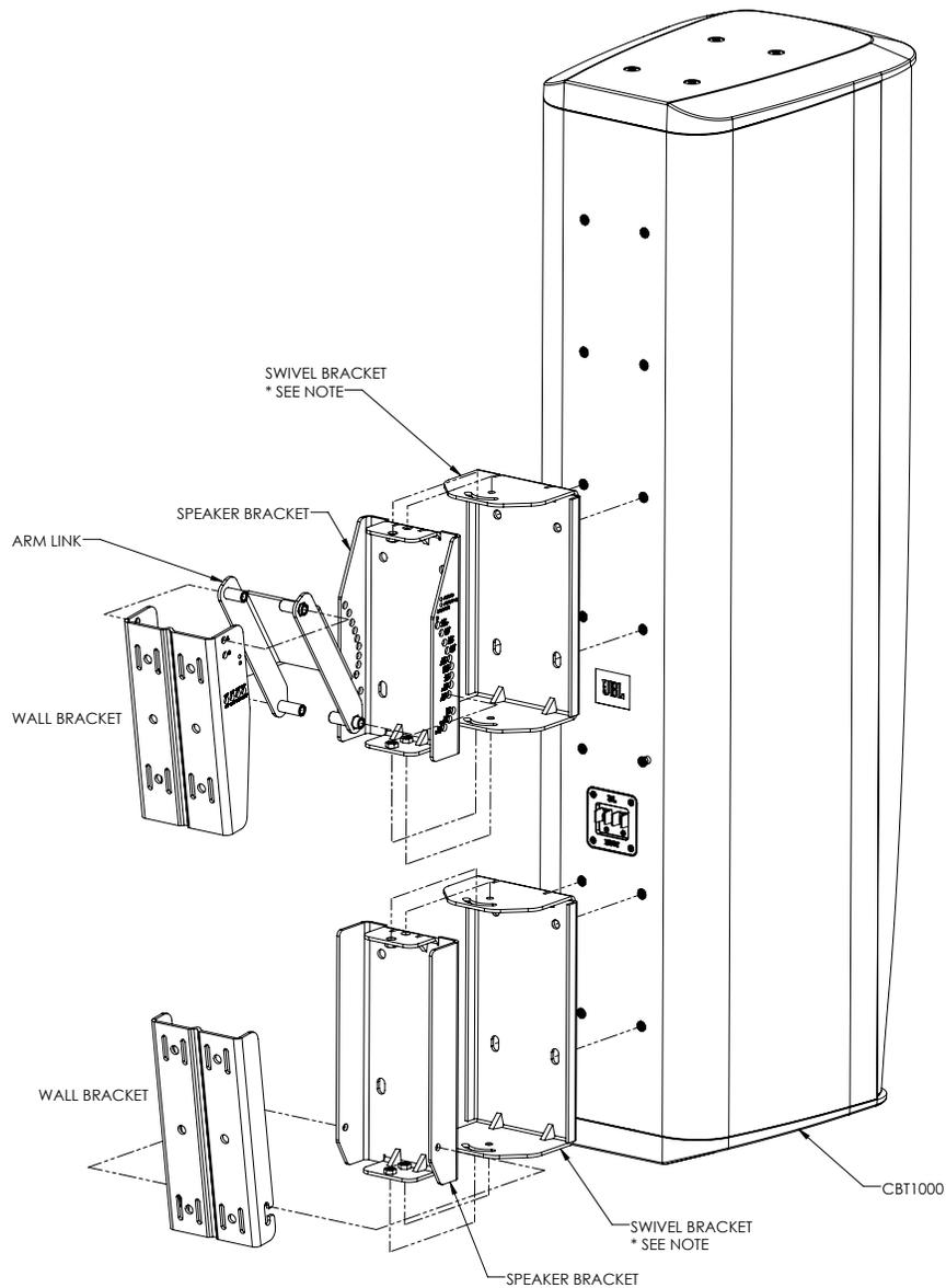
\* NOTE: Use SWIVEL BRACKETS when panning is needed for aiming speaker horizontally. When panning is not needed, leave SWIVEL BRACKETS out, and mount SPEAKER BRACKET directly to CBT 1000 cabinet. Diagram is example only. Consult JBL CBT 1000 Bracket Installation Guide for detailed installation instructions.
