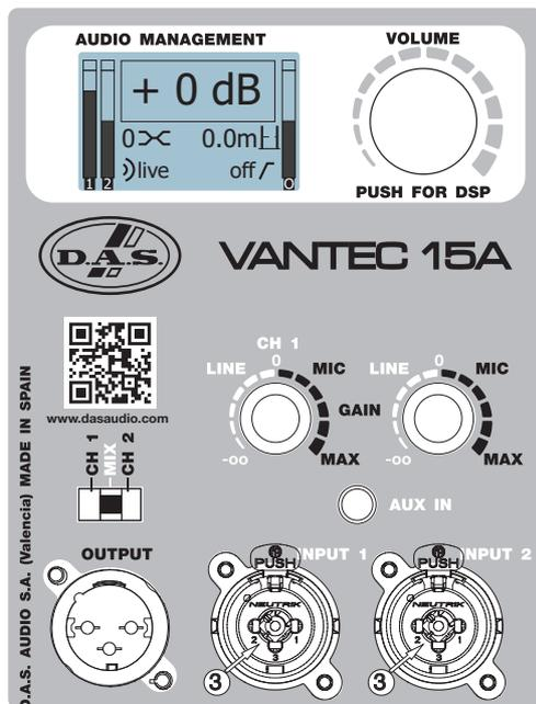
**Vantec 15A input and control panel**
