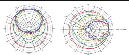
NOTES: Frequency response measured at 4m (13.12ft). For better detail, only light smoothing (1/12th octave) has been used. Polars were acquired by placing the unit on a computer controlled turntable inside a 411  $\,\mathrm{m}^3$  (14514  $\,\mathrm{ft}^3$ ) anechoic chamber. Measurement distance is 4m (13.12ft).
