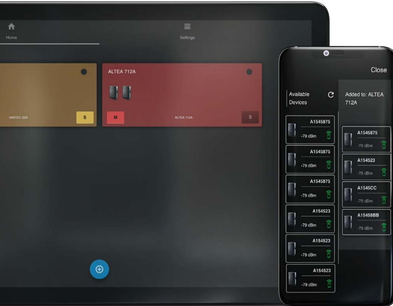
The **Control panel** section is used to simultaneously manage all the systems included in each group and can modify the gain, select presets, perform a customized 3-band equalization, select the number of units and even select the HPF when using subwoofers.
