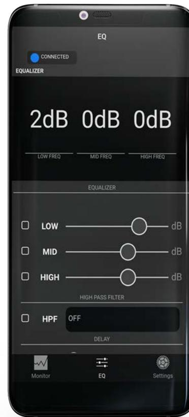
**3** Input and output levels can be monitored using the DASlink™ APP. Super fast set-ups can be done using the presets option. Presets include Live, Dance, Vocals, Bass Boost and Monitor.
