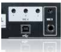
Dual microphone input with independent adjustment
