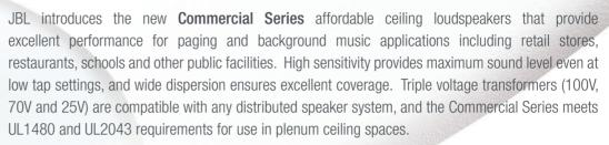
The drivers all feature a full 25 mm (1 in) diameter voice coil with a Kapton™ coil-former and high-temperature wire for superior power dissipation and long-term reliability. The driver, grille and transformer come pre-assembled for ease of installation. Accessories include matching Commercial Series pre-install back cans and tile rails.
